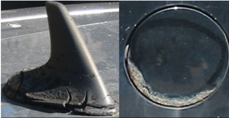
Shark's fin aerials and fuel filler flaps can deteriorate
