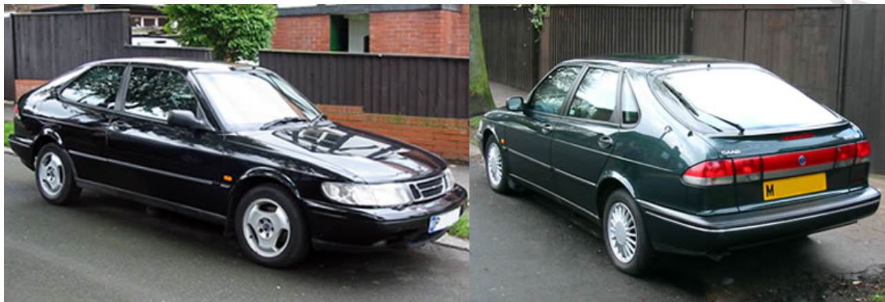
Three and five door variants of the SAAB NG900. The 3 door is a 1996 2.0i 16v 5 speed manual while the green 5 door is a 1994 2.5 V6 SE automatic. Note standard alloys and decor panel on the V6.
