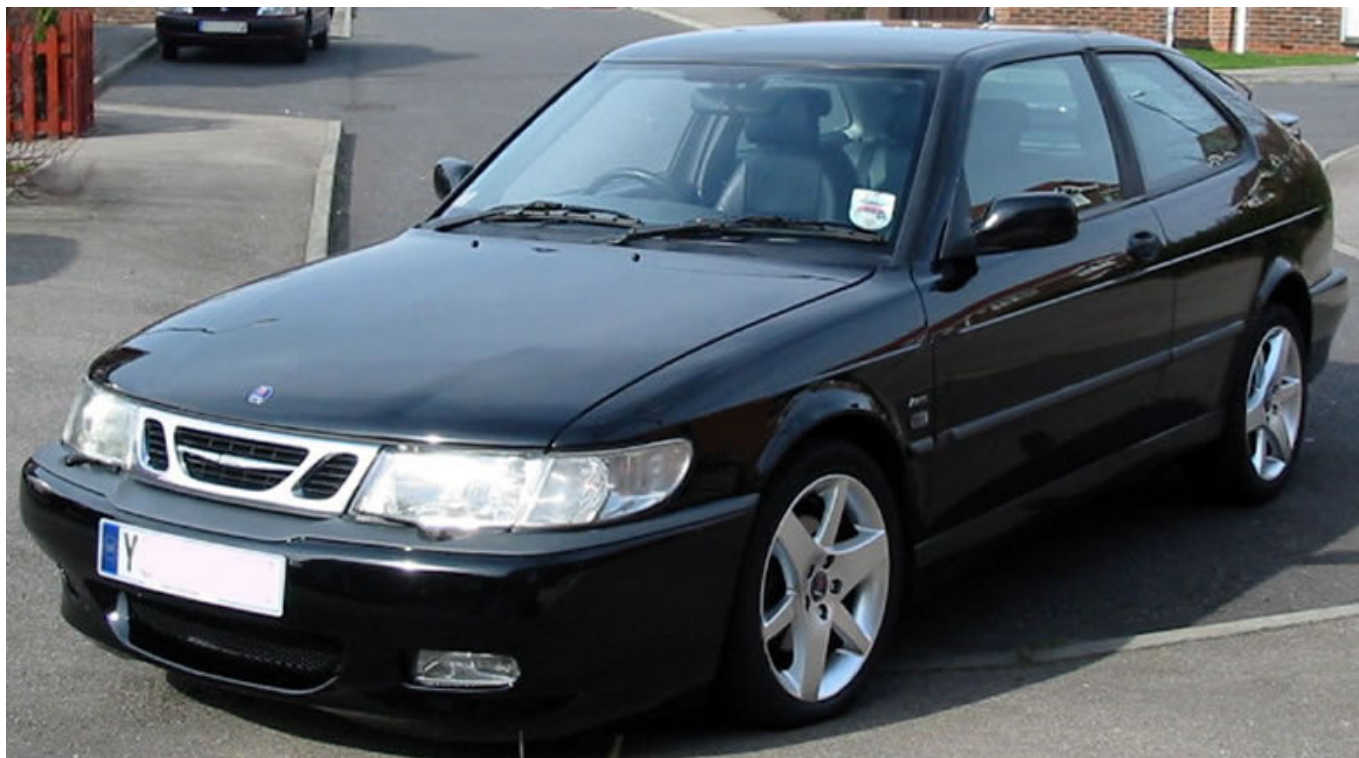
The purposeful lines of the 3 door 9-3 Aero HOT. This particular car, snapped outside the home of the author's brother was a favourite. Note the 17" 'double Y' alloys, lowered suspension, one piece bumpers & side skirts. The 205 bhp engine delivered sparkling performance and 31 mpg in use.
