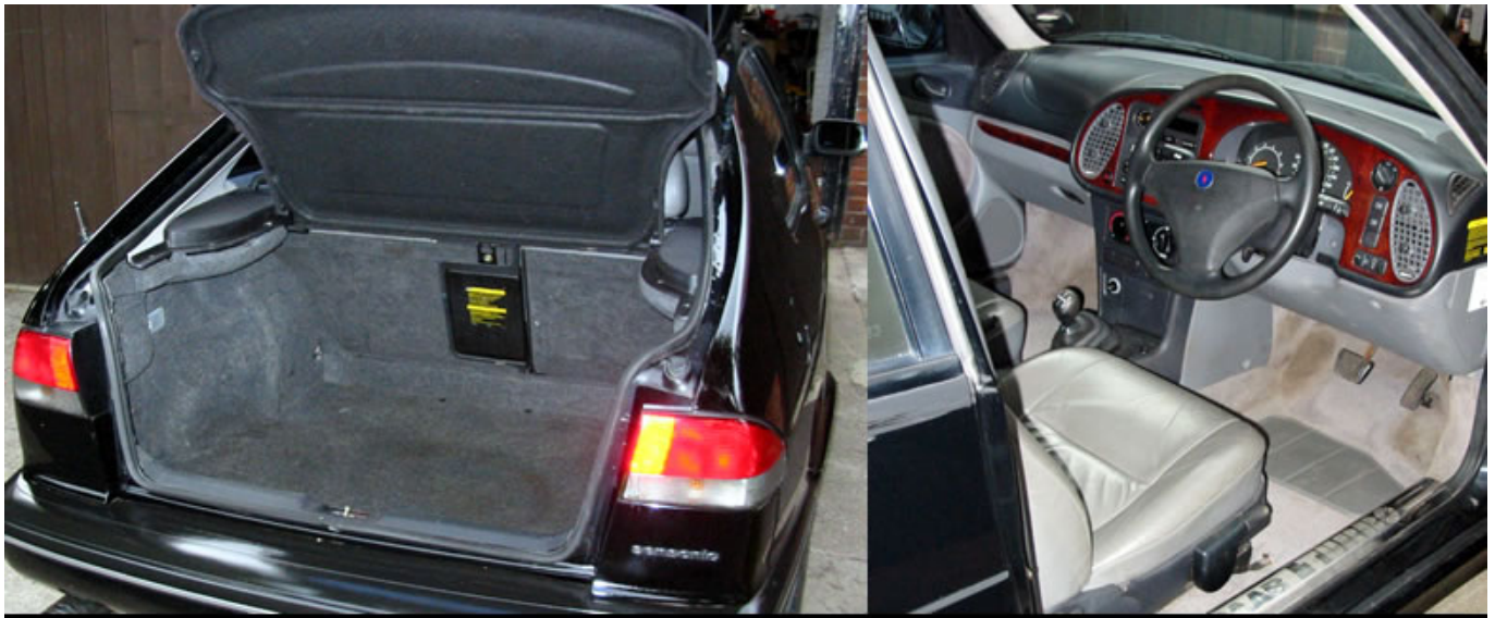
In 3 or 5 door format, the NG900 has good luggage capacity but remember convertibles hold less with the roof lowered! Note the leather trim and wood fascia which were costly options. This car has Sensonic transmission - the system retains the gear lever but dispenses with the clutch pedal.
